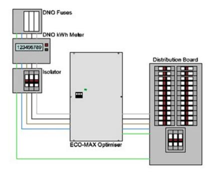
We recommend where possible that the existing earthing arrangement to DB is maintained and a separate earth bond be provided to the optimiser from the DB in accordance with BS7671
