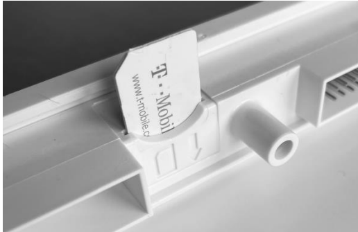
Fig. 7 – SIM card orientation
