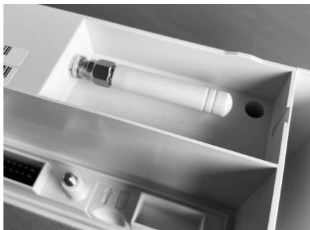
Fig. 5 – Stub antenna fitted to SMA connector
