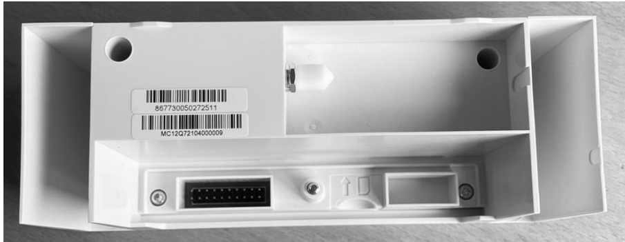
Fig. 4 – Rear of communications module showing antenna housing and SMA connector
