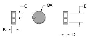
The Round Lead Seal is designed with two parallel holes and a knot chamber. During fitting the wire or string is threaded through the two parallel holes and crossed inside the knot chamber before closing with the sealing tool to prevent slippage.
